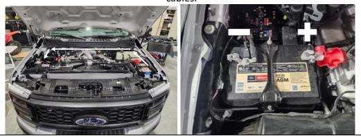
\*Tie all wires away from sharp, hot, and/or rotating components.
