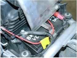
**Step 3.** Once the battery terminal harness has been safely routed towards the front of your bike, you can begin installing the peanut switch and bracket.
