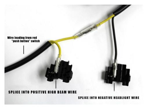
(optional: If you would like to access your LED Lights in low beam or high beam with the red push button switch, splice the yellow coming off the red switch into a key switch constant hot. This will allow you to turn the lights on with the push button switch no matter the stock handlebar switch position.)
