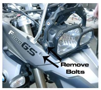
**Step 2:** Once those bolts have been removed, locate the mounting brackets, spacer and reduced flange head bolts which have been included in this kit. Once you have located all of those parts, refer to the drawing below for the installation order.
