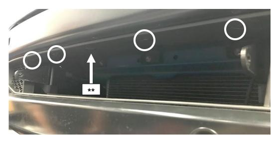
2. Using a Standard screwdriver, pry up the head of the plastic fastener in the grooved portion similar to the image below. Once the head is pulled out from the base of the fastener, the entire fastener can be pulled out. It may require gently prying the base. Repeat for the rest of the fasteners. These will not be used.
