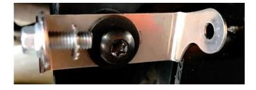
3. With 1 serrated washer and 1 bolt, place into the bracket as shown above. Then partially thread the bolt into the light as shown below. Position power chord as shown below. Once the first bolt has entered the housing, slide the housing up and thread in the second bolt. Using the 8mm wrench, aim and tighten the light. Repeat for opposite side.
