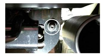
2. Locate the S2 brackets. Using the bolts from step 1 and included spacer, attach brackets on the passenger and driver side in the orientation shown below with spacers under the bracket. Make sure they are level.
