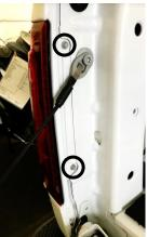
6. With the included Raptor reverse kit upfitter harness in hand, thread the end with a weatherpak plug and an eyelet into the hole behind the tail light and straight down. Make sure the wires exit the body and hang from underneath the vehicle.
