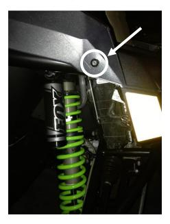
4. Now, at the front of the vehicle, locate the two pressed in black plastic fasteners near the front corners of the hood opening that secure the grill assembly. Using a standard screwdriver, pry up the center section until it appears as shown below.
