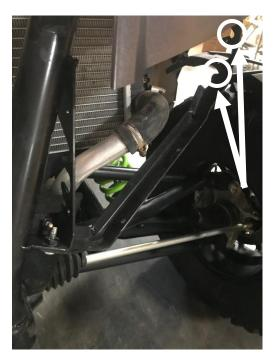
13. Fasten each headlight to the vehicle with the provided ¼" bolts, washers, and nuts in the configuration as shown below. The external faces of the headlight bracket are placed onto the internal faces of the headlight opening. Mount the grill temporarily to check the headlight clearance and remove to adjust. Once satisfied, remove the grill and tighten the fasteners.
